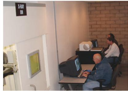
**Networked computers allow students of real-time radiography to conduct annotation of the same image of a casting and, if necessary, send it back for re-inspection. Source: X-Ray Associates LLC**
