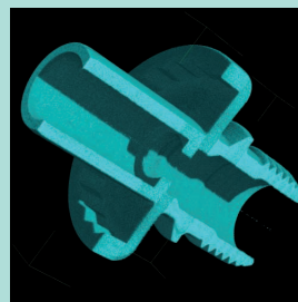
\mu CT of BGA ball (3D view and virtual slice), plastic component, and sensor coil
