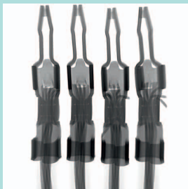
Broken wedge bonds, and crimp connectors
